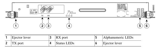
Table 7 summarizes the optics and connectors used by the 1-Port 10-Gigabit Ethernet line card.
